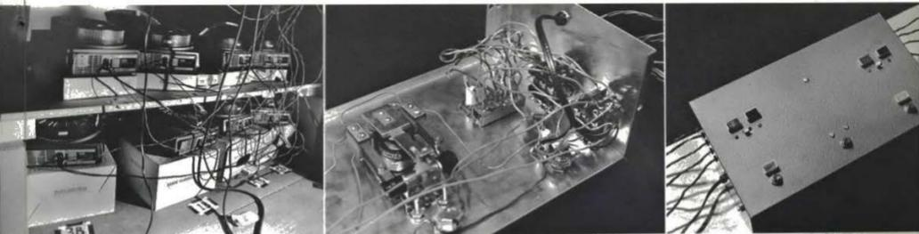
(LEFT) Eight of the ten remote-controlled slide projectors used in the 1968 show. The taped-down numbers refer to screen positions. For this temporary set-up, projector boxes were used as stands. (CENTER) Part of the slide control-box interior. Sequencing relay is on the left. The two relays on the right could change slides in up to five projectors. (RIGHT) Thermostat control box ran two banks of slide projectors. Colored lights indicated switch positions in the dark.
